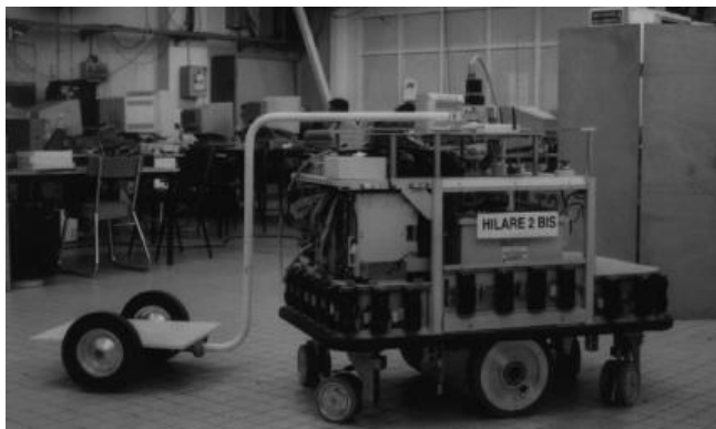
Figure 6: Robot and trailer used in experiments. Reprinted from (4)
